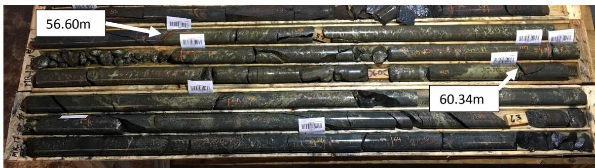
**Photo 1:** Copper & nickel bearing massive sulphides (56.60-60.34m down hole) in drill hole MR-17-01. Disseminated sulphides (20-50%) occur higher in the hole.
